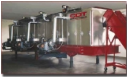
CDT's pilot scale test dryer – 4 ft. x 30 ft. unit
